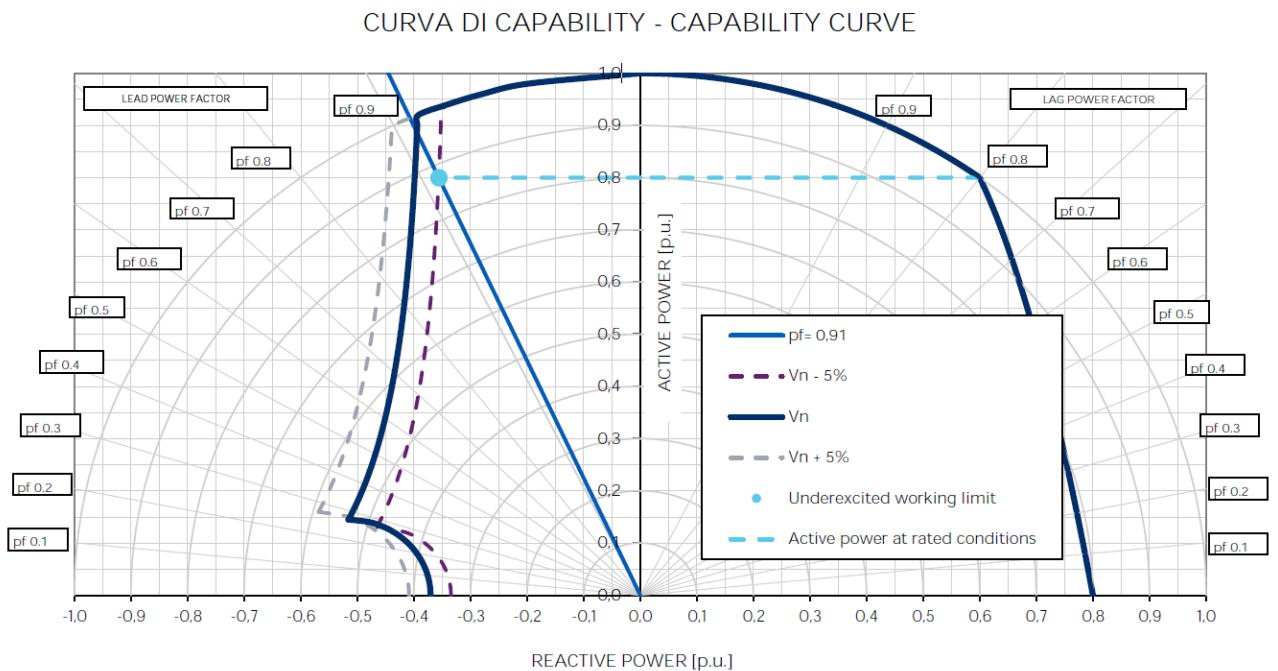
**Figure 1 Generator capability curve**
