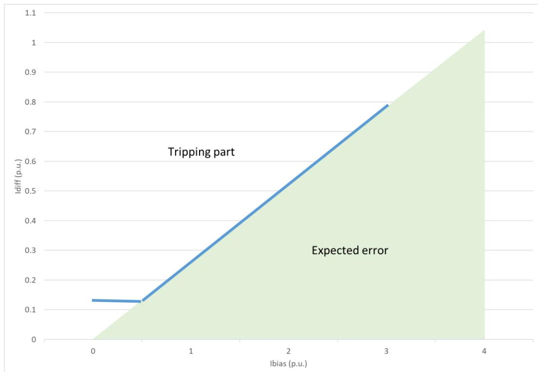
**Figure 5 Differential relay characteristic**
