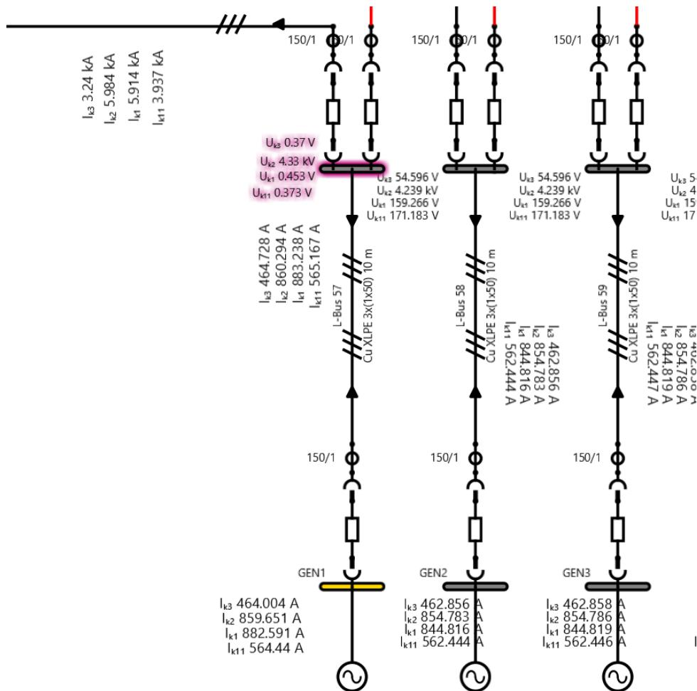
**Figure 2 Short circuit currents: case A**
