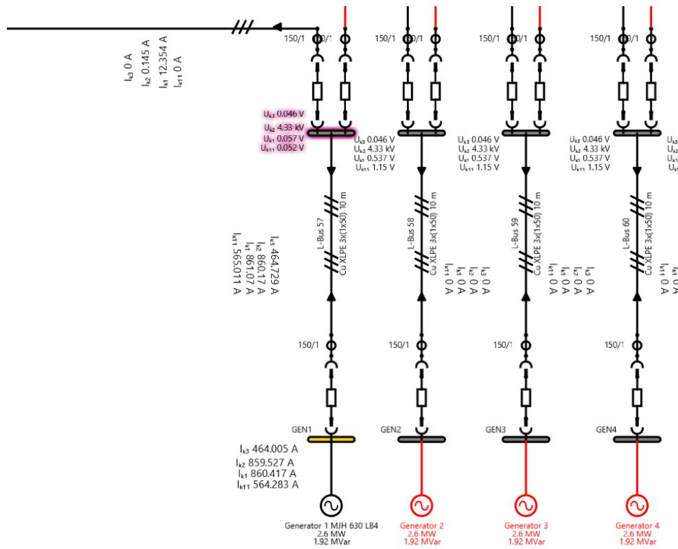
**Figure 3 Short circuit currents: case B**
