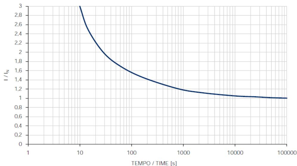
**Figure 6 Generator overload curve**
