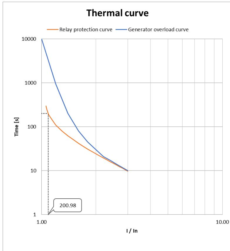
**Figure 7 Generator overload and relay thermal curves**
